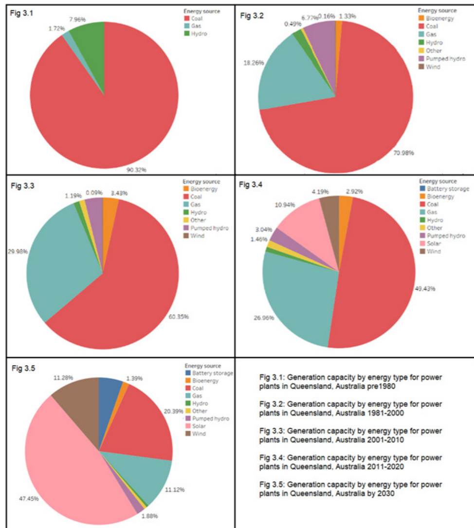
Figure 2. Generation capacity by energy type for power plants in Queensland (pre-1980, 1981-2000, 2001-2010, 2011-2020, by 2030)
